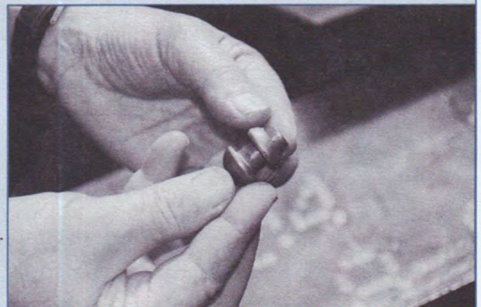
Figure 8. The process of duplicating the appearance of hot rivets began by drilling out the stem of one rivet (shown here on the right) so that it would fit over the stem of another rivet (left).
