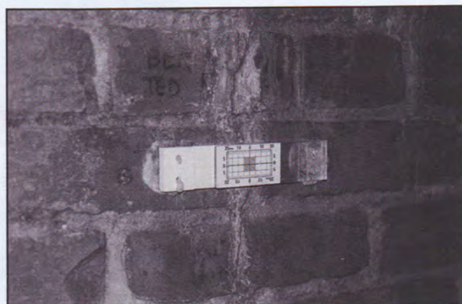
A crack gauge is a useful tool that can help determine extent, rate, and periodicity of movement. Fort Barrancas, Florida.
