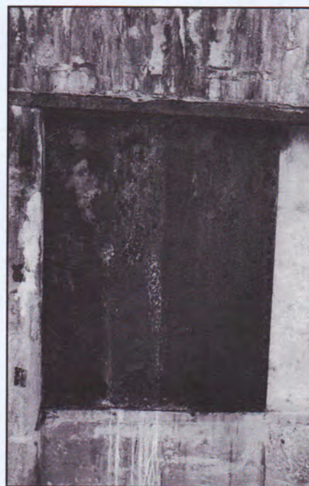
Always test products, especially rust converters. Here, several products are undergoing long-term trials (including one that has left a white residue on the surface) Battery Grattan, Fort Flagler, Washington.
