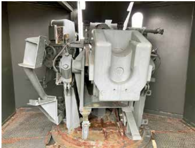
90mm M3 Fixed Mount showing vandalism and serious steel deterioration
