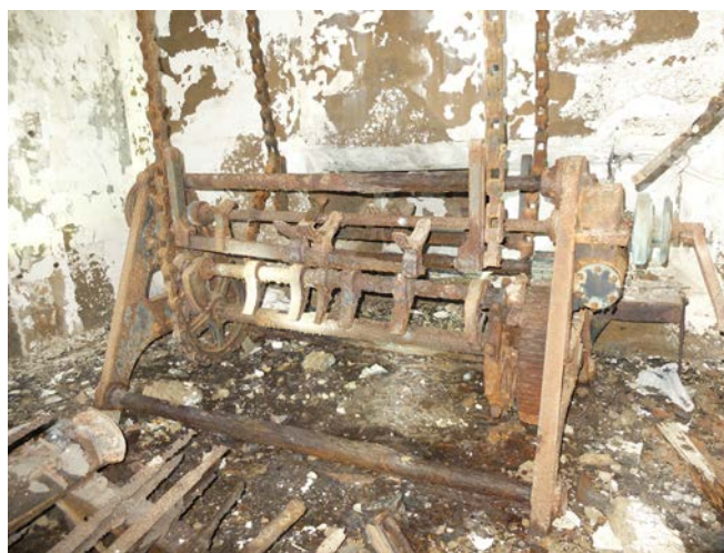
One of three Taylor-Raymond chain hoists in Battery DeRussy. NPS is looking for ways to preserve them. (McGovern Collection)
