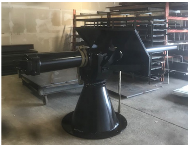
M1898 3-inch gun on a reproduction mount ready to be installed at Battery Smur
