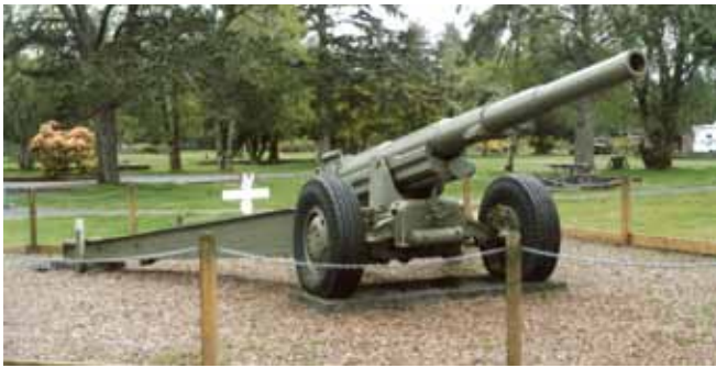
GPF gun at Fort Stevens. Note the "high speed" wheels and tires.
