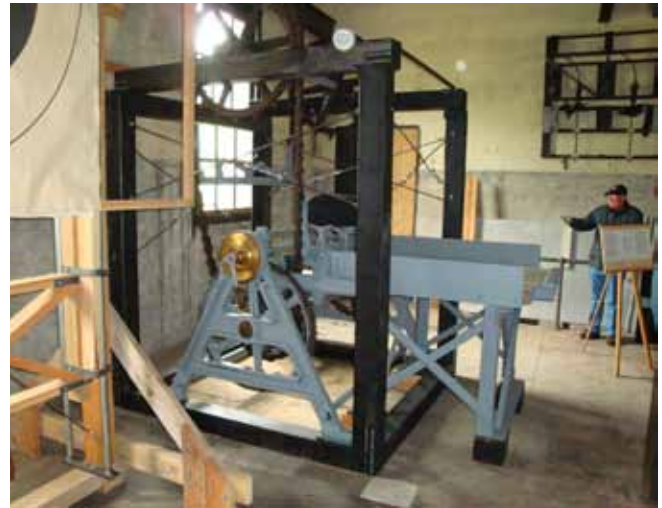
Working mock up of an ammunition hoist, Fort Flagler
