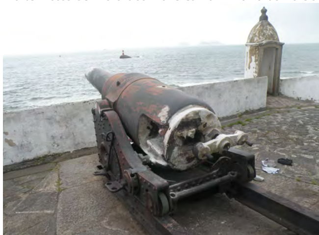
70 pdr (5") Whitworth RBL, an ex-naval gun installed at Paranaguá in 1898
