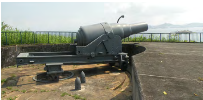
Armstrong 11" RML model 1874 at São Theodosio fort. a ex-naval gun, of the same type used to arm the forts manned by the navy in Rio.
