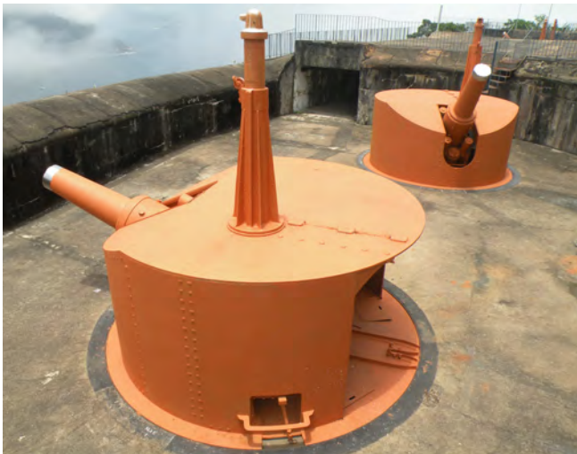
Mortar pit with two Krupp 280 mm L/16 mortars model 1912, their splinter shields is 1" thick. The mast above the mortars houses the back-up depression range finder of each gun.
