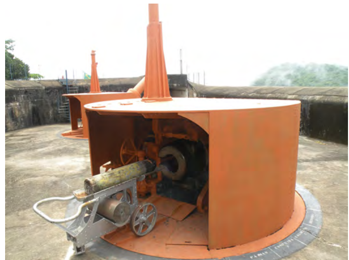
Back of a Krupp mortar, with shell cart and a practice (wood) shell (top) and the cartridge case in the bottom of the cart.
