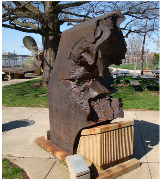
Test fire damage to Japanese battleship armor
