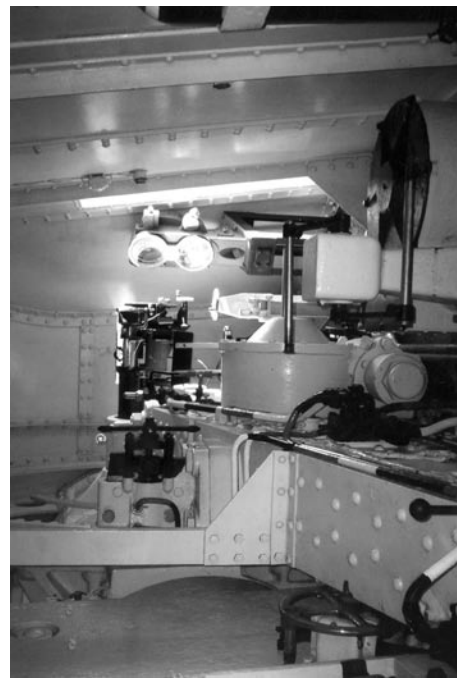
27. The right side of the Camposoto 305 mm gun, looking at the gun trainer and gun captain's positions.
