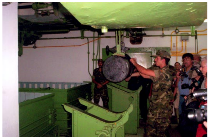
10. The second overhead monorail has picked up the shell from the tray where it was deposited by the first monorail. The shell will now move to the ammunition hoist.
