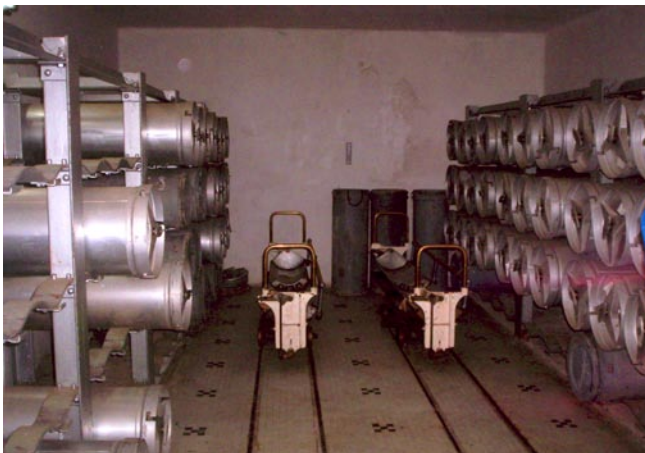
7A & B. The powder room and its metal powder containers. Note the powder carts, the narrow-gauge track, and the tile floor. I understand the powder is removed from the metal containers and placed in one of three carrying containers, standing up right against the back wall. The gunpowder is carried in these containers to the gun.
