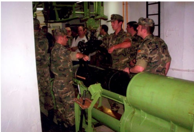
12. The shell being lowered from the second overhead monorail into the shell hoisting mechanism.
