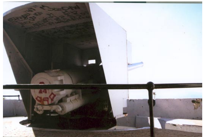
19. The breechblock of Devil's Gap's No. 2 Gun. The interior is smothered in graffiti and the breech welded in place.
