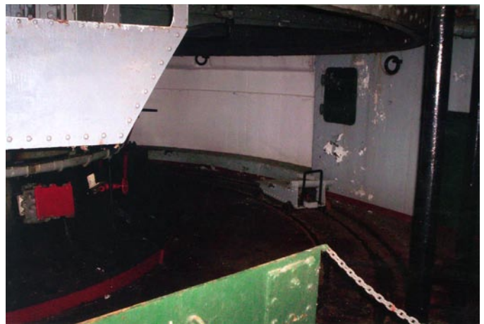
4. Trolley used at O'Hara's Battery to move shells from the ready locker to the loading hoist.
