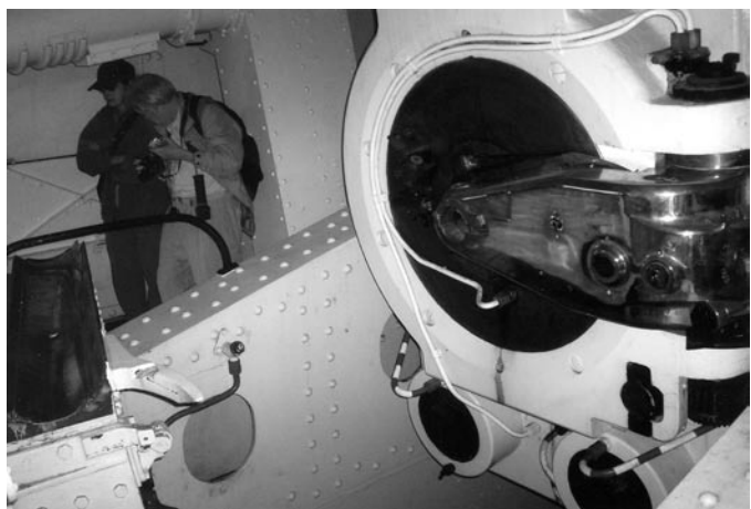
29. The breech of the Camposoto 305 mm gun. In the lower left, the loading tray for the gun is perpendicular to the gun.
