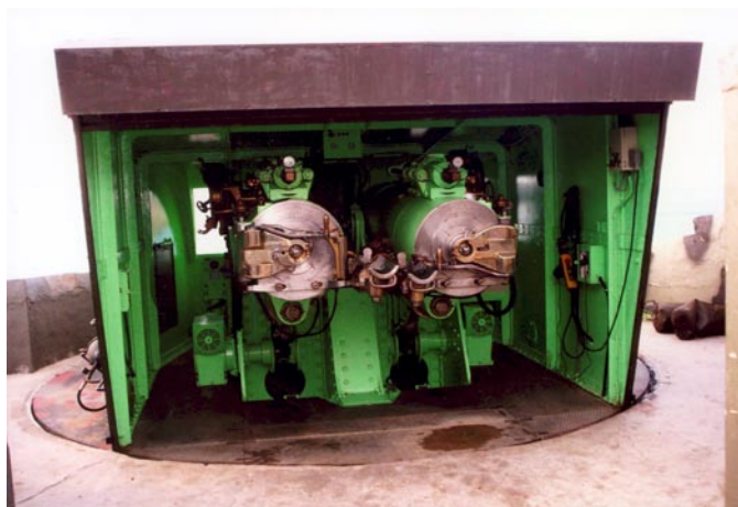
28. The lever for opening the left-hand "V" breech is at the top of the breech, and that on the right gun is at the bottom of the breech.
