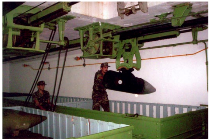
9. The shell has been picked up from the storage bin and is being moved to the next overhead monorail position.
