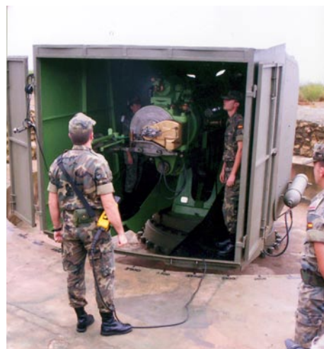
7. "Standby!" is given before firing the gun with the yellow box carried on the side of the gun captain. Note the bearings painted on the rim of the concrete gun pit and the thin shield.
