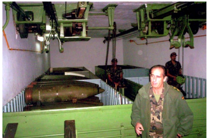
8. The shell room with the shell bins and the overhead monorail. The shell clamps can rotate 360 degrees to grab a shell or deposit it at the monorail that carries the shell to the loading hoist. No one could explain the storage of the shells in the metal bins.
