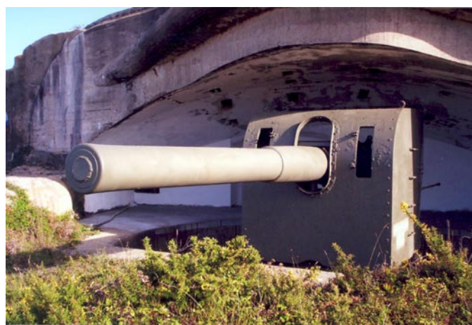
1. A 152.4 mm/50 "W" gun in a covered position near A Cuenca, out of service with the barrel plugged. The shield provides little protection from shell splinters.
