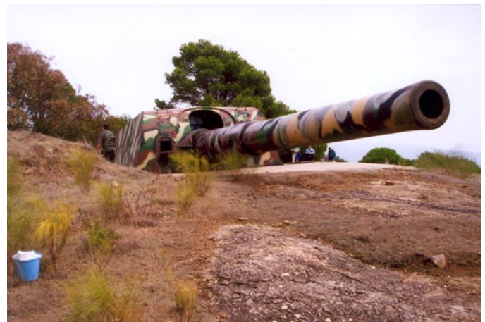
20. A view of the Paloma Alta gun from the front with the barrel depressed. The steel shutter has been removed from the window at the gun captain position (See Illustration 18)
