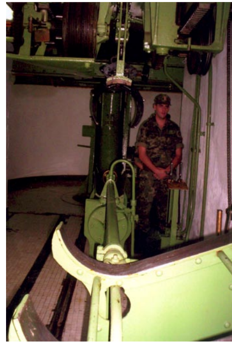
13. The shell raised into the ammunition hoist, starting its journey to the gun.
