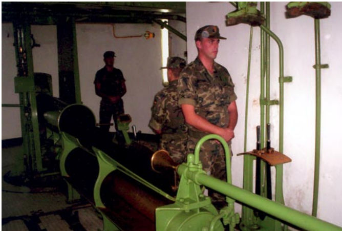
11 A & B. The shell will be lowered into this tray, and the brass cap will push the shell into the shell hoist container.
