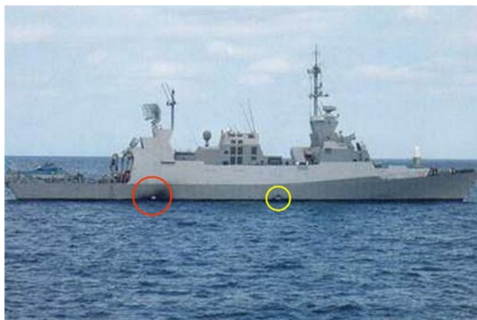
Reported hit location of the C-701 in left circle. Both circles are diesel exhaust for the two diesel engine rooms.
