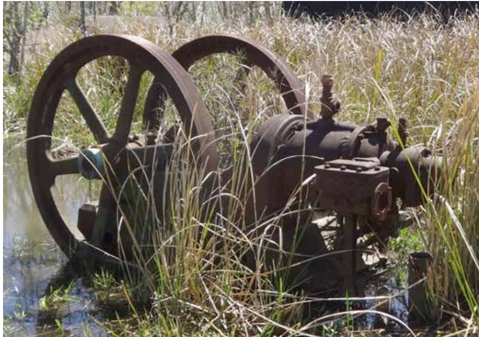
A Hornsby-Akroyd oil engine used for the water pumping system at Fort St. Phillip near Buras, Louisiana
