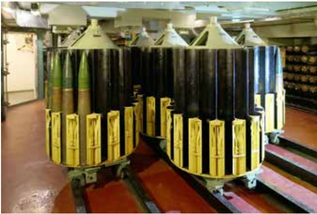
10.5cm m/50 system automatic loading system (CHB)
