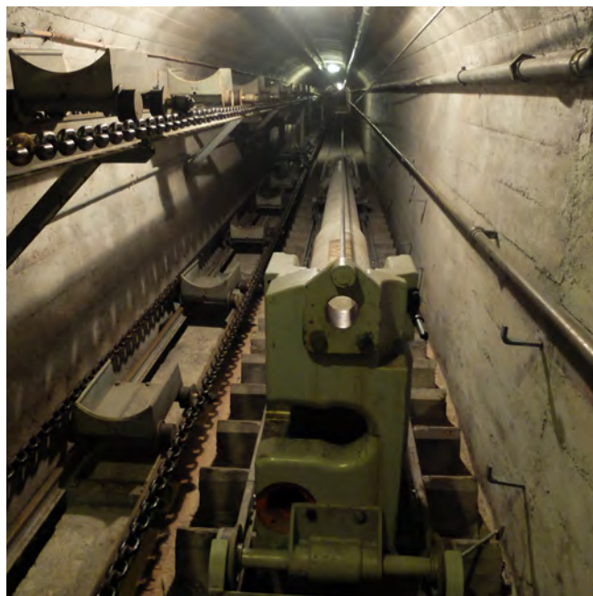
Our guides show us how a replacement 10.5 cm barrel is moved to the turret at Artilleriewerk Magletsch.
