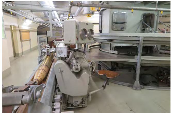
Shell and Casing lift at Battery T1 that elevates up a 160 foot barbette to the gun allowing 15 rounds per minute C. Penfold
