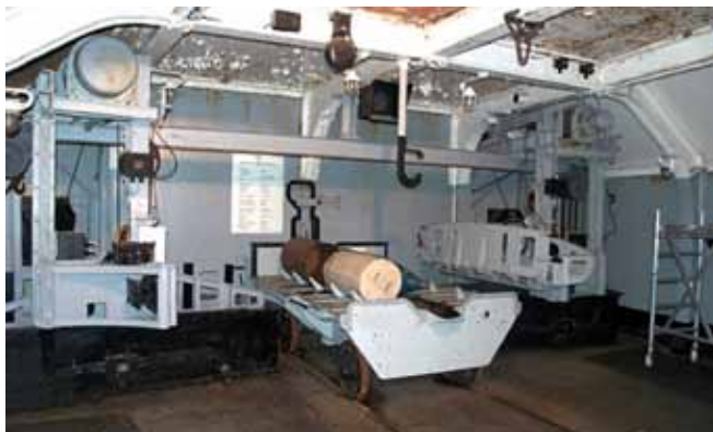
Inside 38cm mount with shell lift, loading table, and air ram for Emplacement #2 at Battery Vara, Movik Fort
