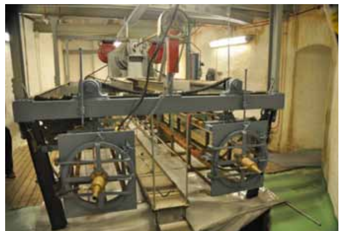
Torpedo Battery – Fortress Oscarsborg – Dual Torpedo Elevator over underwater portals – June 10, 2013
