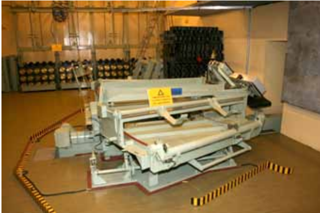
The automatic shell loader for the 12 cm L/70 gun – door behind loader leads to turret
