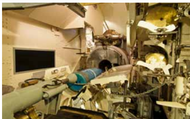
Austrått Fort – Close up of 28 cm SKC/34 gun with shell tray and power rammer
