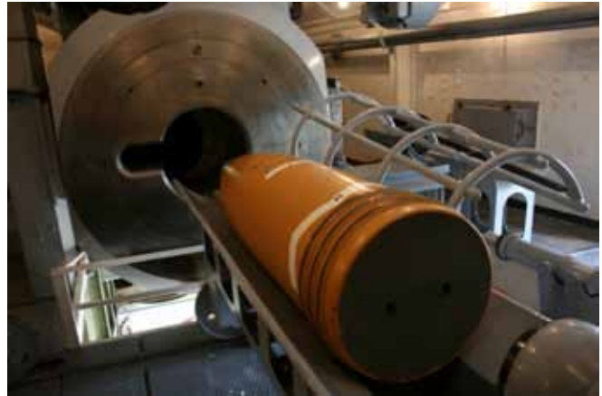
The shell table is now swung into place so the hydraulic rammer can do its job
