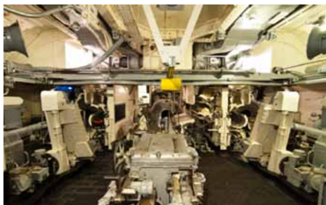
Austrått Fort – Inside the 28 cm SKC/34 triple turret – looking at power rammers and open breeches
