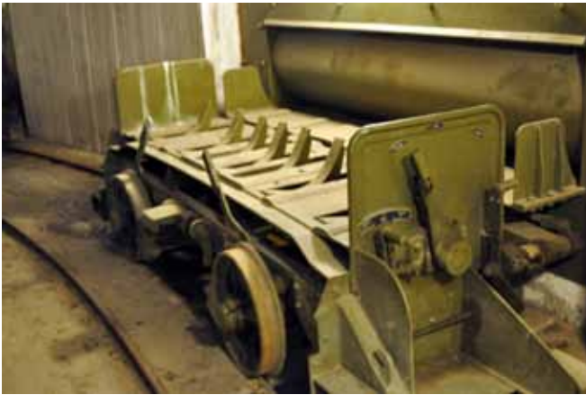
Shell wagon to move projectile to shell lift as the gun rotates to firing position
