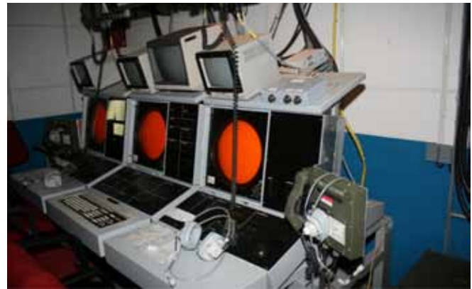
12/70 command and control center – target radars console for each gun
