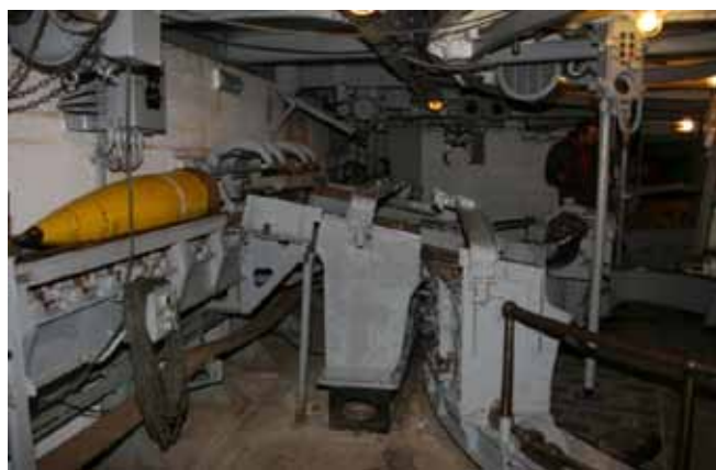
Austrått Fort – Shell handling room 28 cm SKC/34 triple turret that transfers the shell to the lower turret
