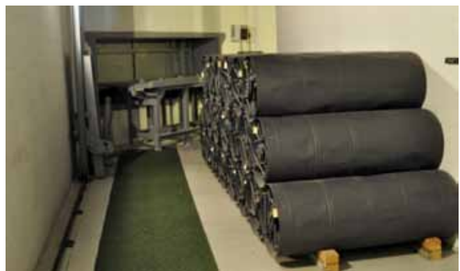
Powder canisters with transfer table in background to move powder to the gun well and lift
