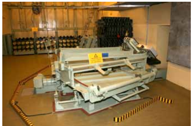
Magazine for the 12 cm L/70 gun – Shell racks, pallet mover, and shell loader
