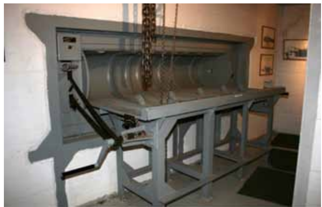
Shell table with overhead hoist to transfer projectile from magazine into gun well – one at a time.
