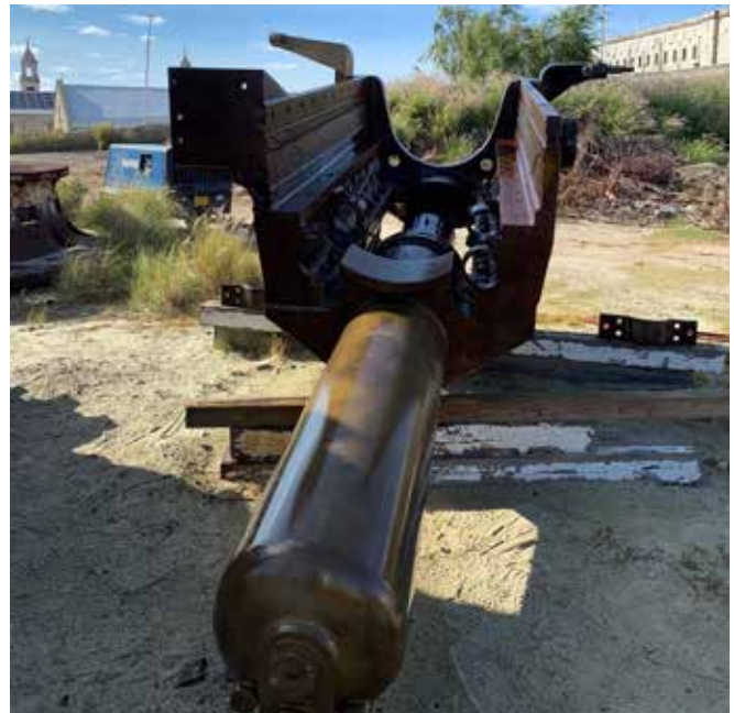
The cradle and recuperator assembly. 10.06.2020 (MT)
