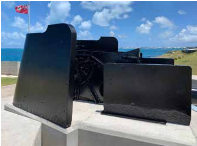
Main shield, side shields, carriage and cradle (MT)
