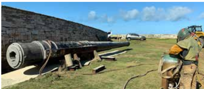
Sandblasting the barrel. 26.3.2021 (MT)
