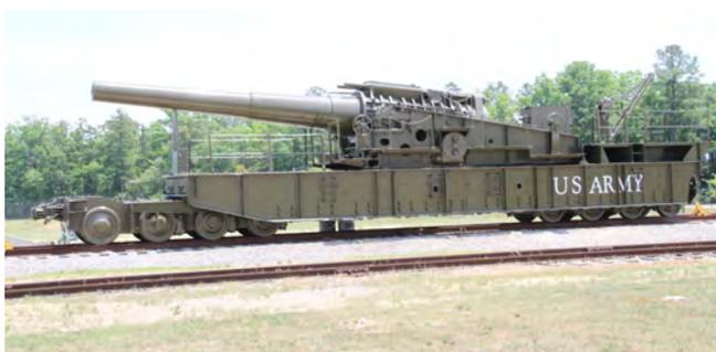
Some minor restoration was done. Several missing stanchions were replaced; others that were bent have been straightened. The contractor also reproduced the chain box for the loading crane and manufactured an authentic muzzle cover. The finished product looks great and can be seen from SR 36 which passes through Ft. Lee. The gun can be viewed up close at any time on the Ordnance School campus. Access to Ft. Lee, VA, is
