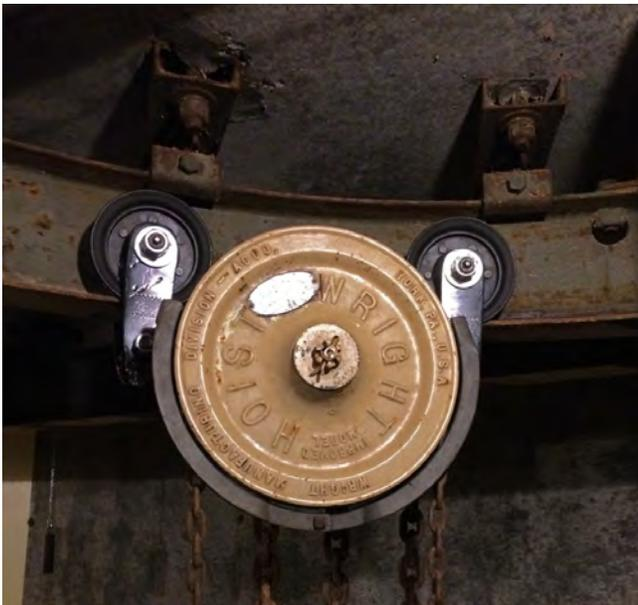
reassemble the dollies, unsnarl the chains, and put the hoist back into fully operating condition. The completed assembly was set onto the overhead rails for display in the projectile magazine. For the first time in over 60 years, there's a fully operational trolley inside Battery Townsley.
